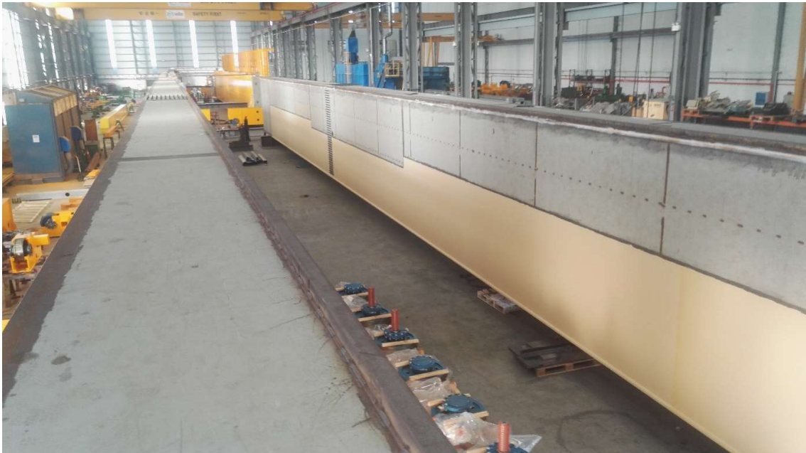
Figure 1 Girders for a unit of 40m overhead crane
