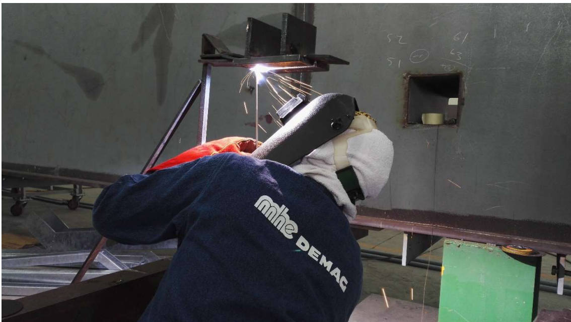
Figure 2 Welding of welding procedure qualification test specimen at the 4G welding position
